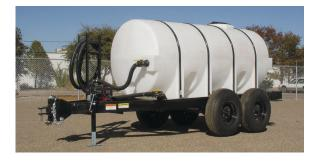
The **1025 Full Drain Tandem** nurse trailer is designed for transport of water, liquid feed and liquid fertilizer. Constructed of 6" channel iron, tandem slipper spring axles, polyethylene tank, pipe hoops to secure tank to trailer, heavy duty six hole wheels, and four implement tires.
