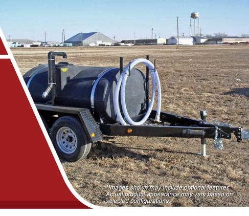
The 550-Gallon Express Potable Water Trailer is designed for easy delivery of potable water to remote sites like RV parks, cabins, portable offices, and temporary facilities. Built with an algae-resistant tank, food-grade components, and a DOT-approved trailer frame, this unit delivers clean water where you need it, fast and hassle-free. Its gravity-fed design uses three hose bibbs and a 2" outlet for efficient discharge without requiring a pump.
